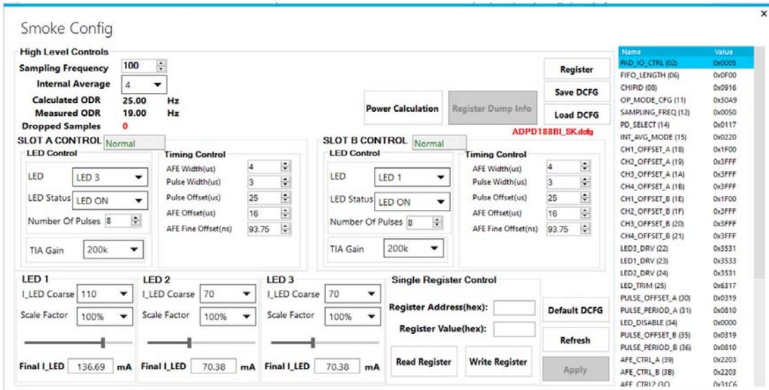
Figure 18. Smoke Device Configuration (**Smoke Config**) View
