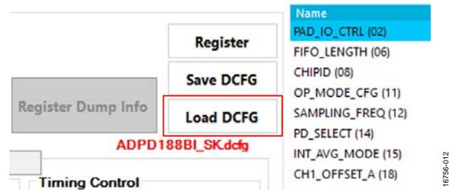
Figure 12. Selecting **Load DCFG** to Select the Configuration File
