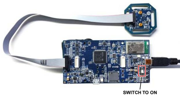
Figure 3. Connecting the EVAL-ADPDCUZ to the EVAL-ADPD188BIZ-SK
