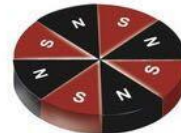
單面扇形充磁 Sectors on One Surface Magnetised
