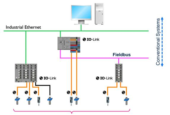
IO-Link → Communication Down to the Sensor / Actuator
