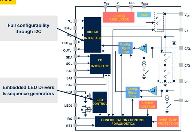
Configurable switches, very low  $R_{DSON} = 2\Omega_{max}$
